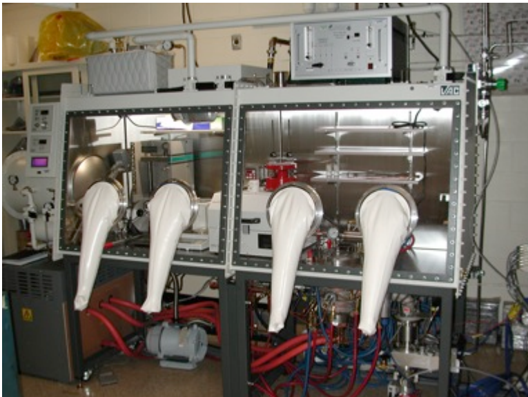
Glovebox with pressing and sintering capabilities
