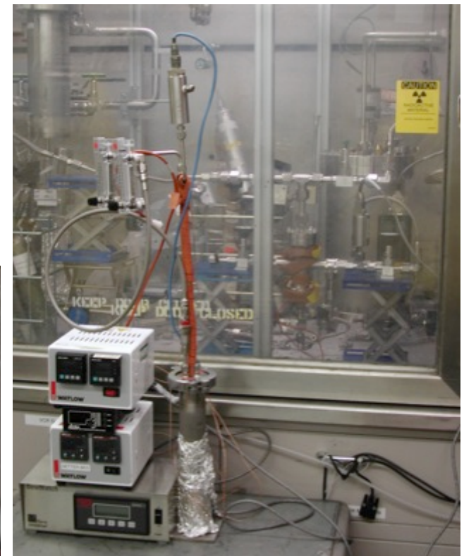
Reactor (in hood) and humidifier (front) for \text{UO}_2 synthesis by IDR route
